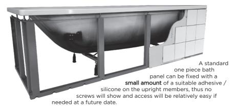
If however a tiled finish is being planned, the board can be fixed by drilling a pilot hole first and then a coated self tapping screw. Another method would be to use a suitable adhesive/silicone to adhere a tile-backer/waterproof cement board on the upright frame members, tiling can be finished thereafter. An access panel can easily be achieved (as shown below) by tiling outwards from Upright ONE. for full details on this please see our online video
